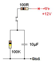
When the push switch is released, estimate how long it will take for the capacitor voltage to drop to 6 volts.
