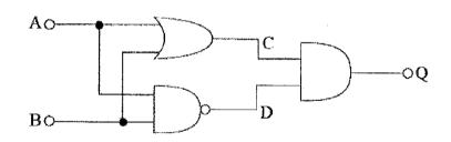
Complete the truth table below to show the operation of this logic circuit.
