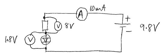
In the circuit above, the battery voltage is 9.8 V. The LED voltage is 1.8 V. The LED current is 10 mA. Calculate the value of the resistor.
