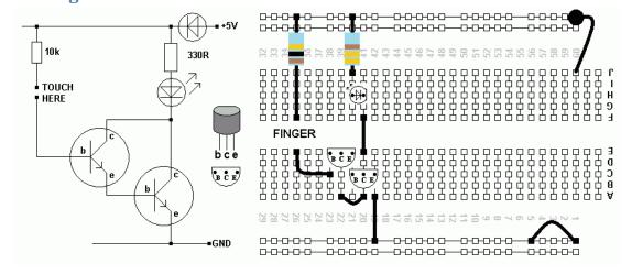
This uses two transistors so the current multiplying effect is much greater. So great in fact that just touching the base connection without completing the circuit is enough to light the LED. Your body is acting as an antenna and picking up all the electrical noise in the room. This is sufficient to light the LED.
